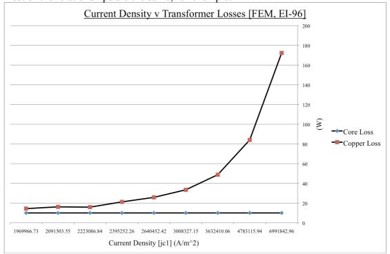
This graph should be equivalent to the top right graph in fig 3 produced by Matlab. The efficiency however does not follow the same relation. This comparison is inadequate as the changing current density in simulation 1 was due to a change in geometric proportions that doesn't occur here. That proportion is a significant variable so it's likely it will be responsible for discrepancies between results. FEMM
