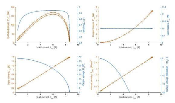
These graphs show performance standards for the transformer with a changing load current. During the first assignment we were changing the proportion ks, as this ks increased the current density (jc1) decreased. This current density is roughly proportional to the load current so we can compare data from assignment 1. Most of the relationships are the same, for example:
