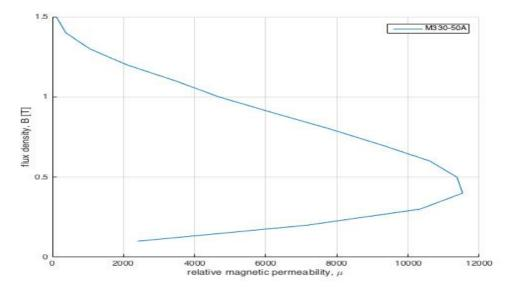
The data in this graph is for a 0.5mm sheet of steel; an iron transformer core will have a higher saturation rate so 1.4T would be a more suitable choice for that metal. A lower flux would be more power conservative but generally the higher the permeability of the core, the more efficient the transformer is.
