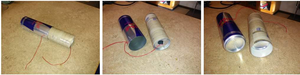
Figure 9: Practical realization of a can capacitor.
